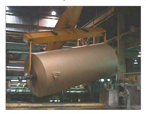
We can prevent accidents like the one pictured above by performing frequent and periodic inspections on cranes and below-the-hook lifting equipment. Frequent and periodic inspections are defined in ASME B30.20 Below the Hook Lifting Devices, while crane inspections are defined by other industry standards such as CMAA Spec #78. Lifting beams come in many different configurations, but inspections are very similar.
