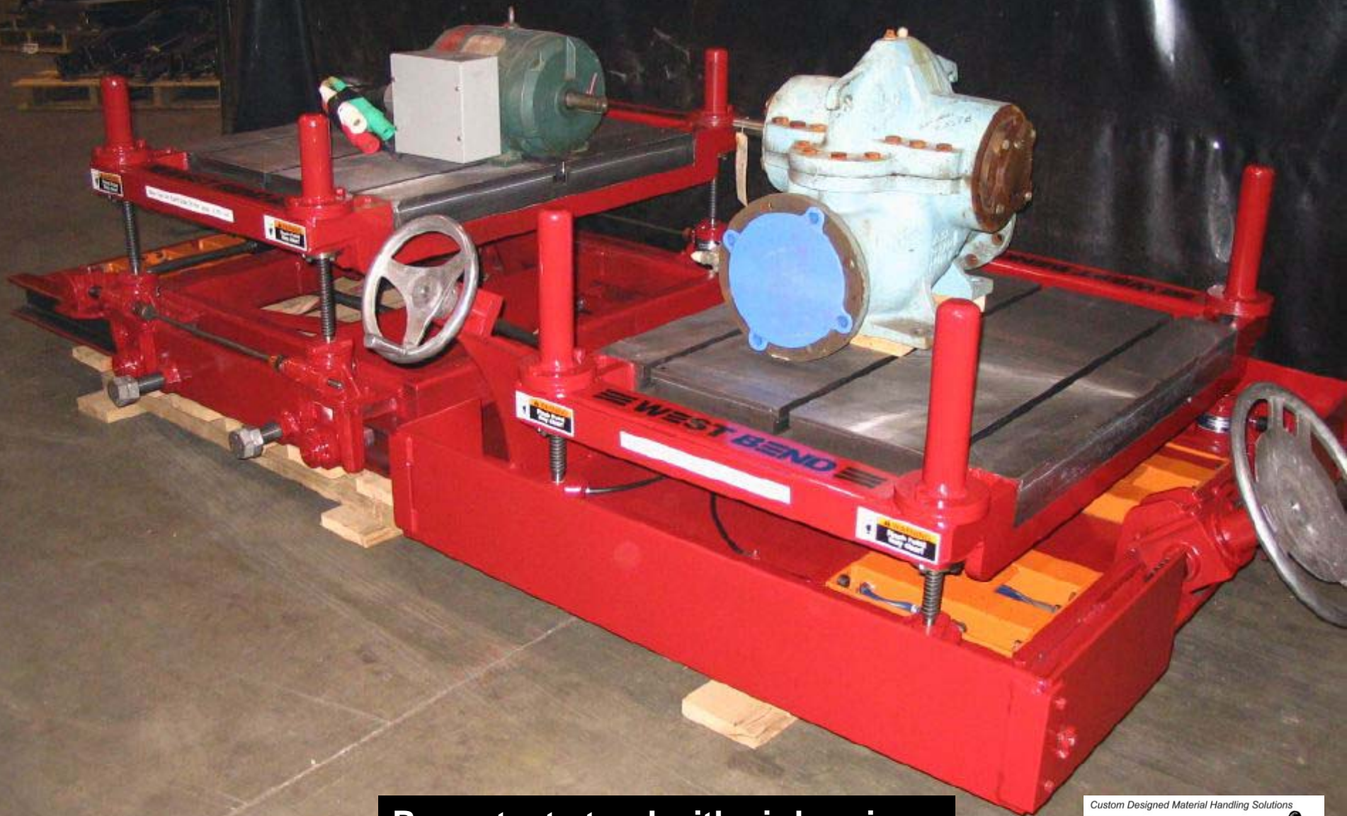
Pump test stand with air bearings
