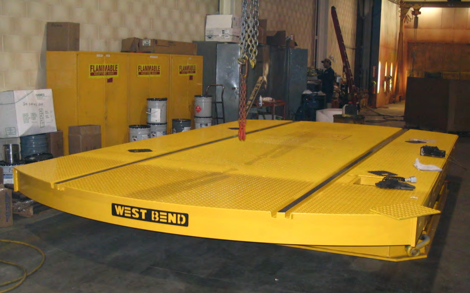
Floor turntable for locomotive component assembly
