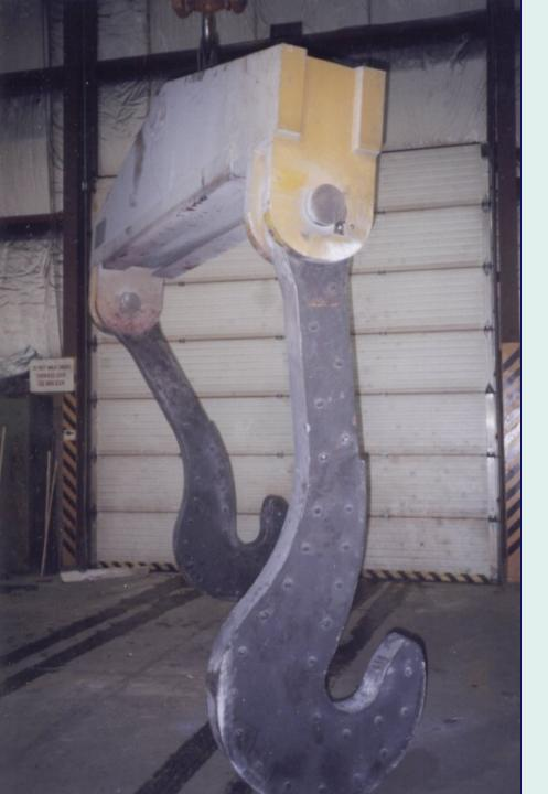
Beam with single-direction pivoting hooks.
