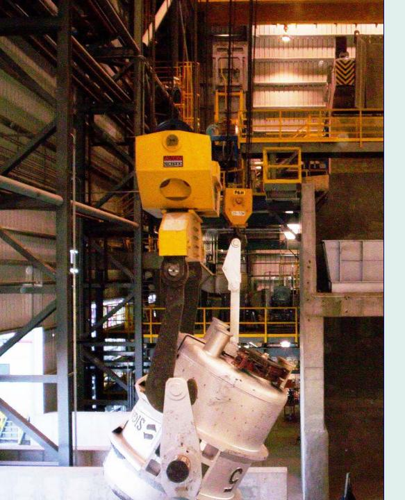
Ladle beam with motorized rotation
