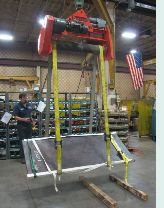
Metal plate inspection- Use Flip-Rite® to inspect underside
