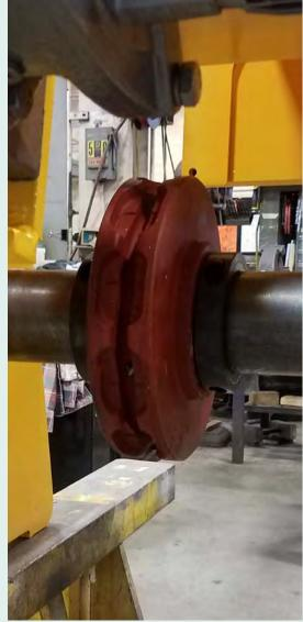
Flip-Rite® modules with pocket wheel for lifting chain
