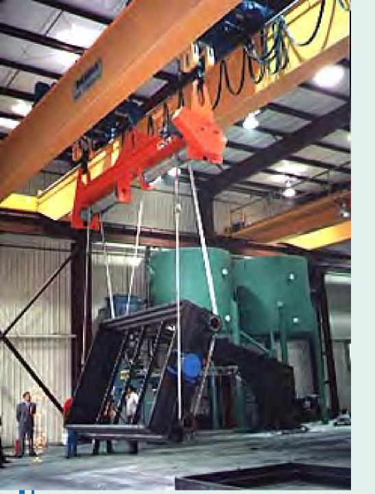
Flip-Rite® in foundry for flipping mold boxes
