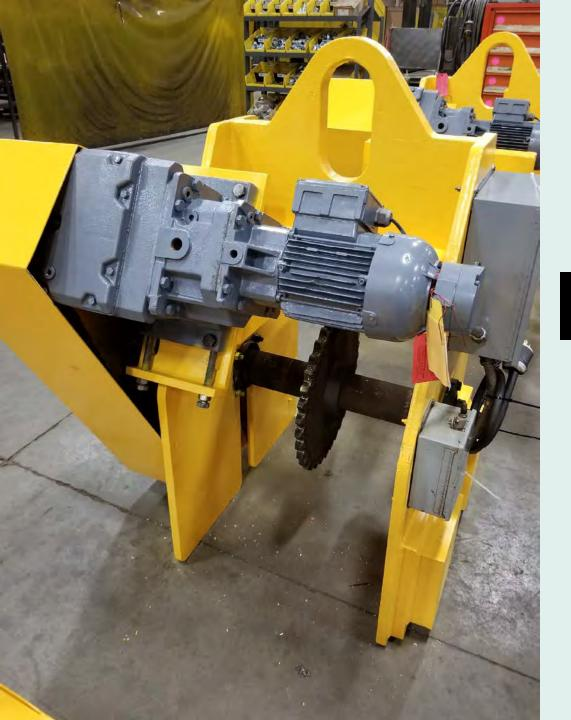
Flip-Rite® modules with sprocket for roller chain
