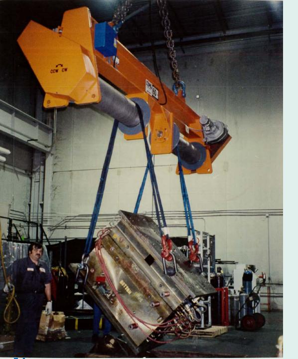
Flip-Rite® for flipping plastic injection molds for maintenance
