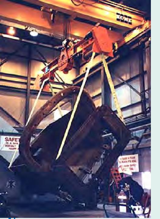
Flip-Rite® for heavy weld repair shop
