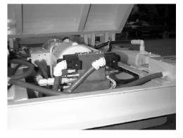
The solenoid valves are located, as shown at right, in the center of the end of the short platform. It should be possible to reach into the machine to gain access to the solenoid valves, even with the platform fully lowered.
