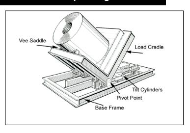
and pivot ears form the "pivot point" of the upender. One or more double-acting hydraulic tilt cylinders are used to rotate the platforms through 90 degrees. Usually the blind end of the cylinder is attached to the base frame, and the rod end is connected to crank ears, mounted on the upending cradle.
