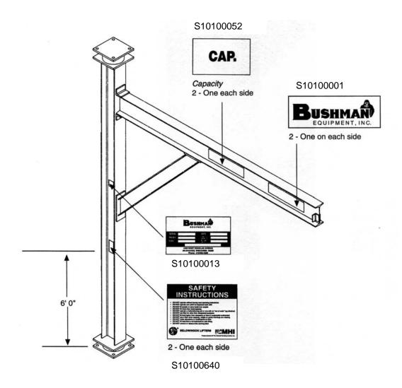
All safety decals must be kept clean and legible and replaced when necessary. Call or send an email to Bushman Equipment to obtain free replacement decals.
