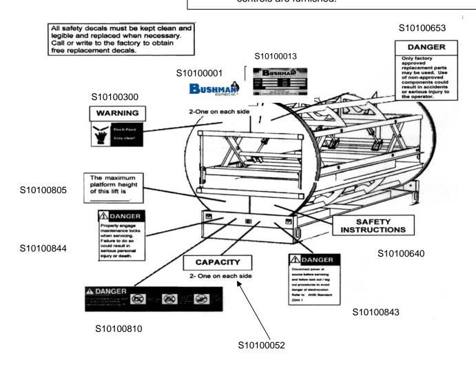
All safety decals must be kept clean and legible and replaced when necessary. Call or send an email to Bushman Equipment to obtain free replacement decals.
