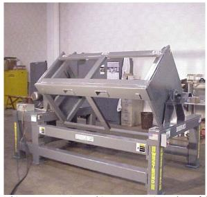
This custom engineered inverter can tip and carefully discharge castings onto a conveyor that runs below it. The capacity of this inverter is 4,500 pounds.
