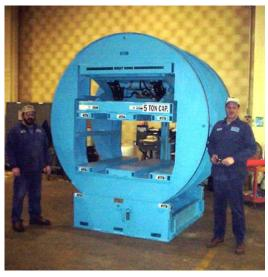
This barrel load inverter has fork pockets built into the platforms. Capacity is 10,000 pounds.
