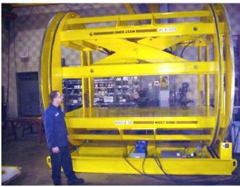
This barrel-style load inverter was designed to invert stacks of aluminum sheets for the automotive industry. The aluminum sheets are inserted and removed from the same side. A clamping force of 5 to 1 prevents the stacks from shifting.
