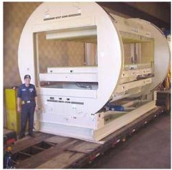
The capacity of this large barrel-type load inverter is 15,400 pounds. The dimensions of the load/unload platforms are 79 inches wide by 180 inches deep.
