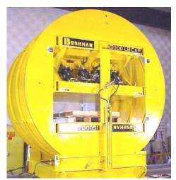
This 15,000-pound capacity barrel inverter, designed for an aluminum blanking facility, includes hydraulic clamping. Adjustable clamping pressure for various loads is an important product protection feature.
