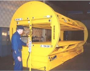
Bushman AvonTec's 5,000-pound capacity barrel inverter features open sides for flow-through sheet inversion. Using a forklift, operators can feed sheets up to 88 by 250 inches into the barrel inverter and remove after inverting.
