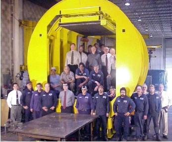
This 5,000 pound barrel inverter has powered roller conveyors to move loads into and out of the inverter. The 60 by 112 inch platform accommodates many of our associates as they pose with the finished inverter.
