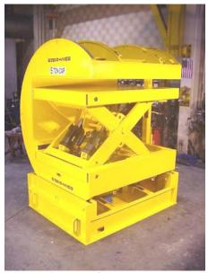
This Bushman C-frame inverter was designed for high capacity, high cycle operations. An industrial gear motor drives rotation on machined wheels that roll on permanently lubricated bearings. C-frame inverters are PLC-controlled so they can easily be integrated into automated process lines.
