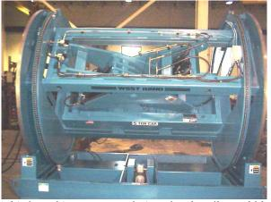
This barrel inverter was designed to handle steel blanks that are unbanded and oiled. The capacity is 10,000 pounds. The load/unload platforms are 94 inches wide by 36 inches deep.
