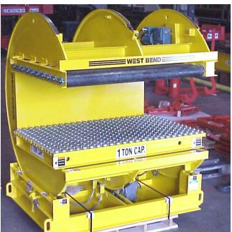
Hydraulic clamping allows materials to be inverted quickly and securely with this C-frame inverter. After rotation, the inverted material can move in multiple directions on ball transfer rollers.
