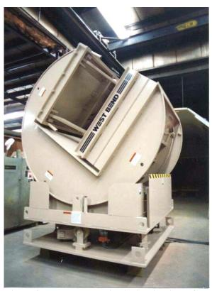
This C-frame inverter with a hydraulic clamp features horizontal rotation for returning loads to the point where they were loaded. Base rotation eliminates extra forklift movements.
