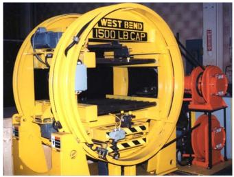
A variety of operations can be performed with this barrel inverter. Features include powered rollers for conveyor-fed process lines and networking with production control systems.
