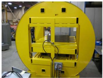
This custom-engineered 180 degree barrel-frame-inverter has a capacity of 8,000 pounds. It was designed to rotate steel blanks up to 63 inches square by 19 inches high. The welded steel inversion cradle is mounted on four machined steel bogey wheels with lubricated roller bearings.
