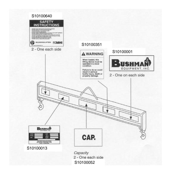
All safety decals must be kept clean and legible and replaced when necessary. Call or send an email to Bushman Equipment to obtain free replacement decals.
