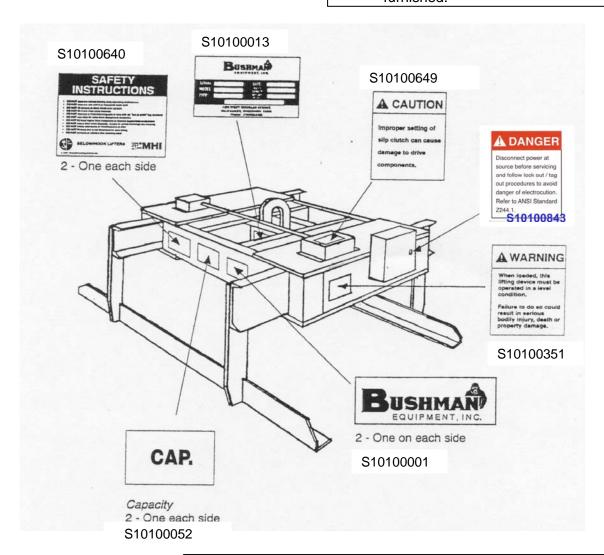
All safety decals must be kept clean and legible and replaced when necessary. Call or send an email to Bushman Equipment to obtain free replacement decals.
