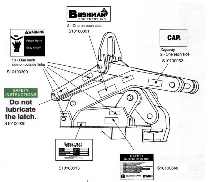
All safety decals must be kept clean and legible and replaced when necessary. Call or email Bushman Equipment to obtain free replacement decals.
