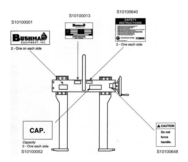
All safety decals must be kept clean and legible and replaced when necessary. Call or send an email to Bushman Equipment to obtain free replacement decals.
