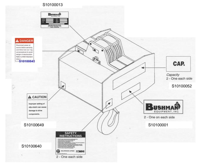
All safety decals must be kept clean and legible and replaced when necessary. Call or send an email to Bushman Equipment to obtain free replacement decals.
