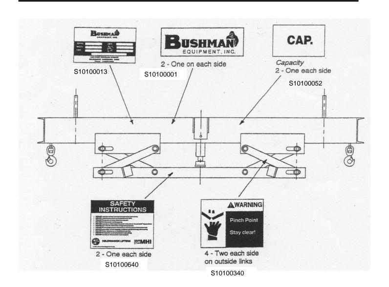
All safety decals must be kept clean and legible and replaced when necessary. Call or send an email to Bushman Equipment to obtain free replacement decals.
