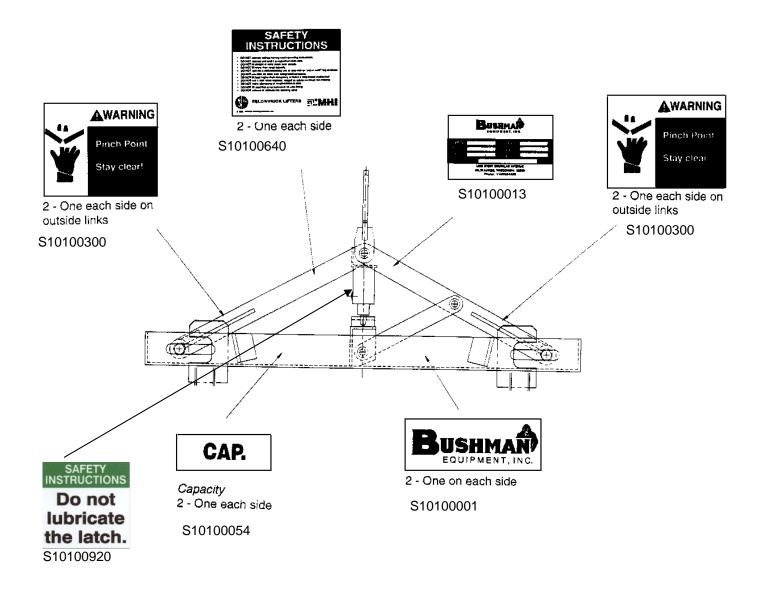
All safety decals must be kept clean and legible and replaced when necessary. Call or write to Bushman Equipment to obtain free replacement decals.
