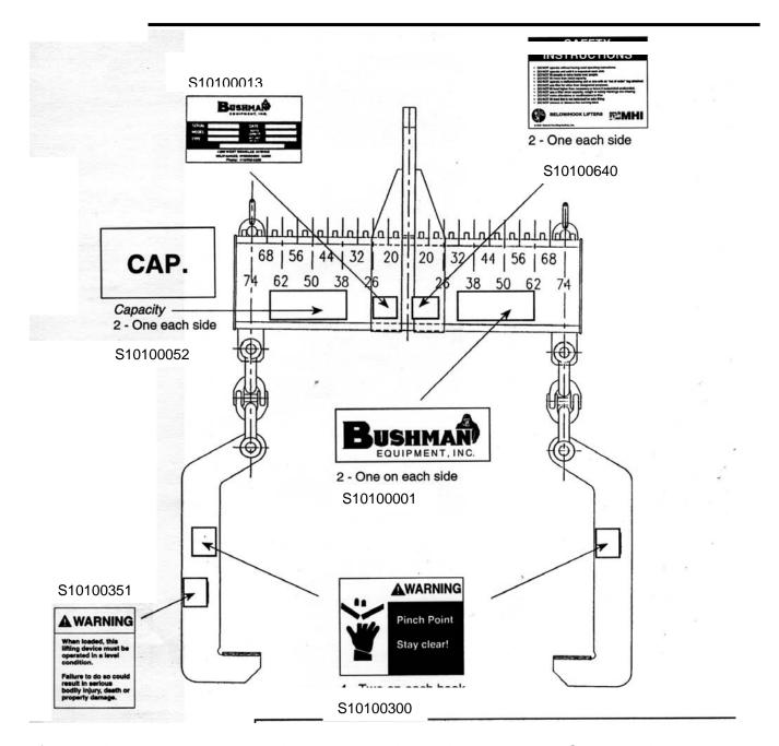
safety decals must be kept clean and legible and replaced when necessary. Call or send an email to Bushman Equipment to obtain free replacement decals.
