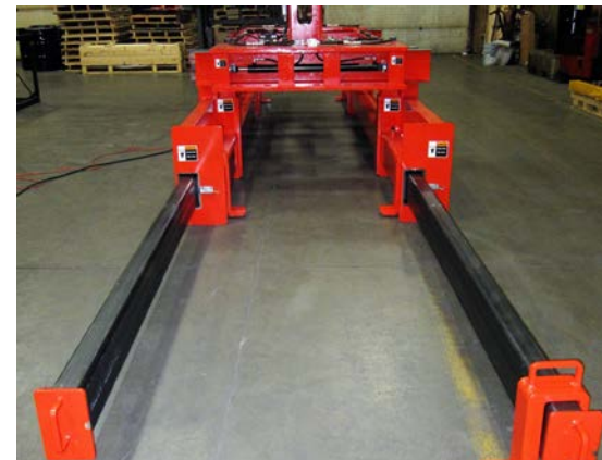
Adjustable forks for varying pallet/bundle lengths
