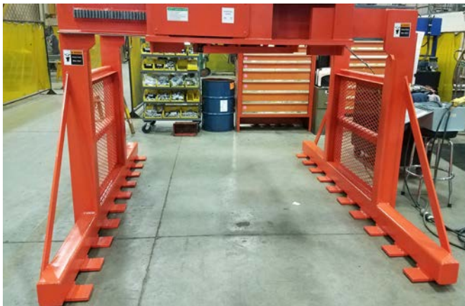
Fixed forks to match pallets or conveyor
