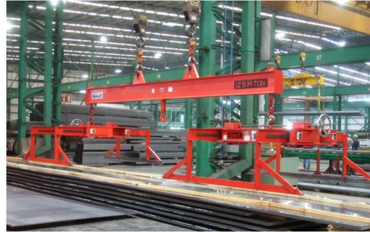
Twin manually-operated sheet lifters can be supported by a spreader beam to lift extra long plate bundles.
