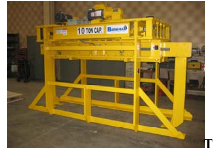
This lifter has two sets of motorized legs to secure the sheet stacks on all four sides.
