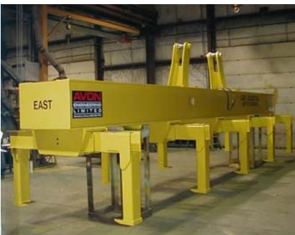
This telescopic plate lifter has rack and pinion design. This 40,000 pound capacity, mill duty lifter has a two-point crane suspension. It can handle plates up to 146 inches wide and 40 feet long.
