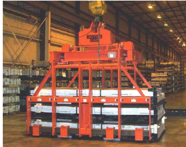
This 30-ton pin-pallet lifter has adjustable forks to conform to different pallets and motorized rotation for efficient loading of trucks.
