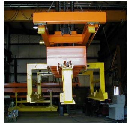
This fully automated sheet lifter is permanently attached to the crane. It also features motorized end supports to reduce the effect of bellying on thin gauge materials.
