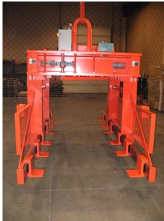
This sheet lifter with adjustable position lifting feet operates somewhat like a fork truck. The feet can be adjusted to fit various loaded pallets.
