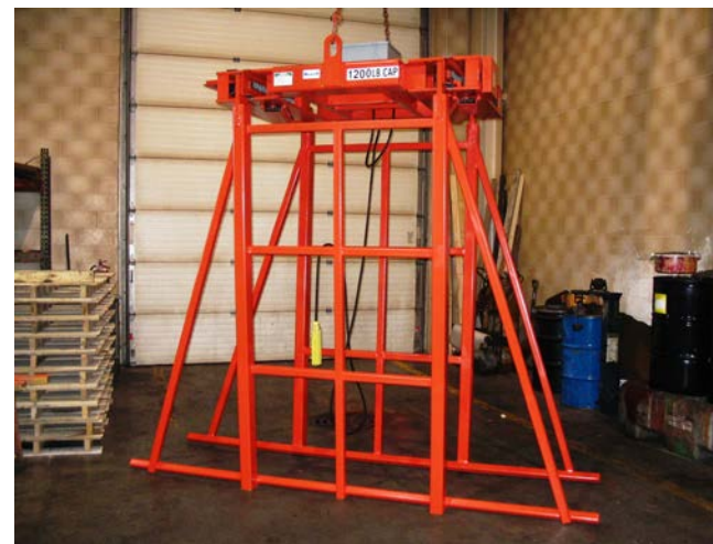
A sheet lifter can be adapted to handling foam buns which are used to manufacture air filtration products
