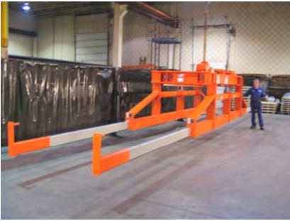
25,000 pound capacity sheet lifter with telescoping carrying arms. Four leg extensions can be manually extended to 40 feet overall length.
