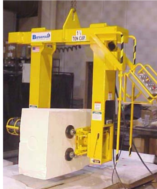
Lifting refractory blocks required grip pads made from conveyor belt material and four satellite pads to spread out the gripping force to prevent the block from crumbling.
