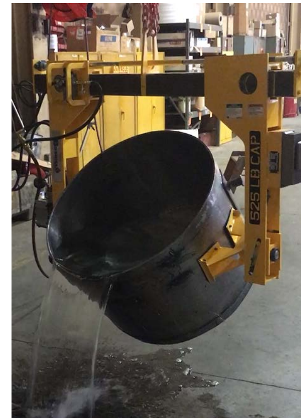
Lifter legs are operated with a hand chain wheel. Rotation is by a hand lever with locking detents.
