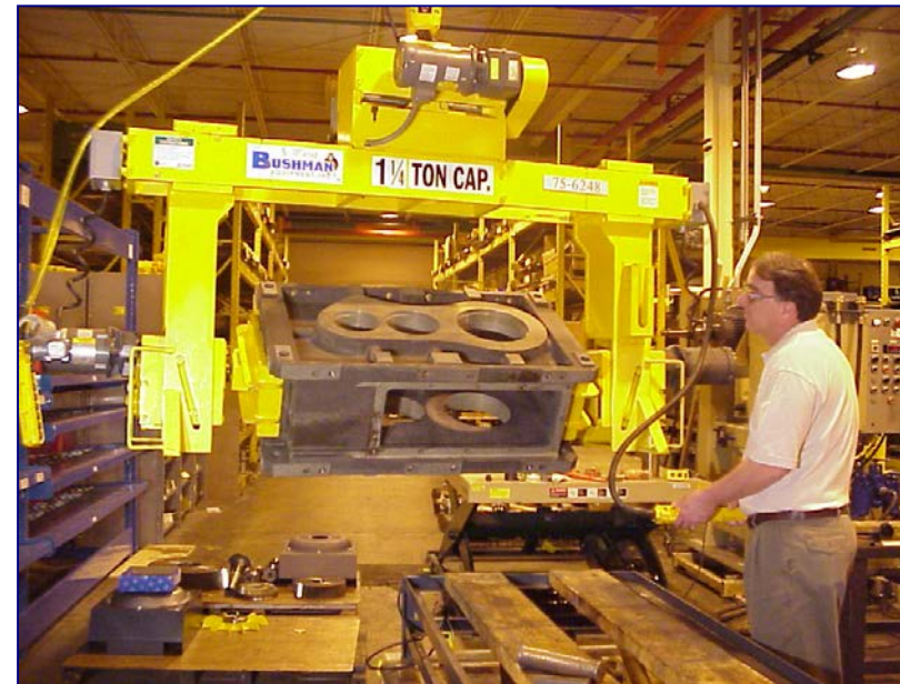
(Above) All motions are motorized. The bail adjusts to maintain level as the load CG changes while the gearbox is assembled.
