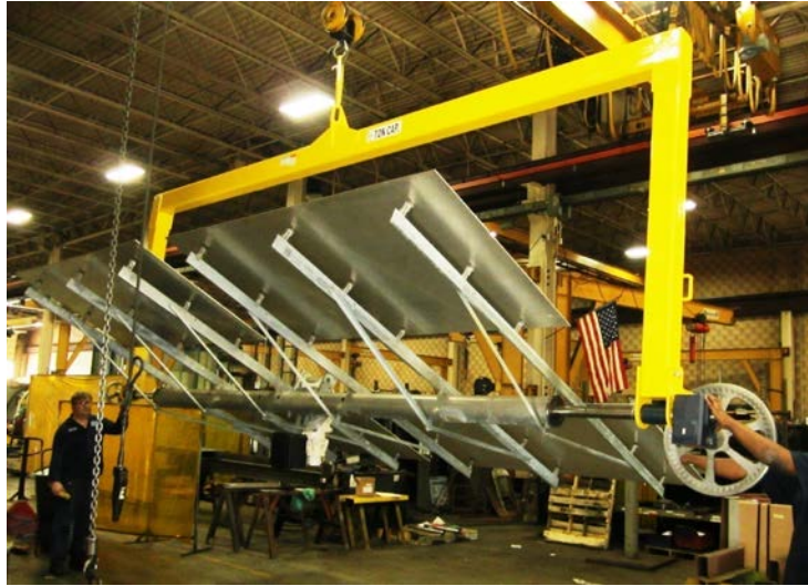
Grab with fixed-position legs picks up solar reflectors
