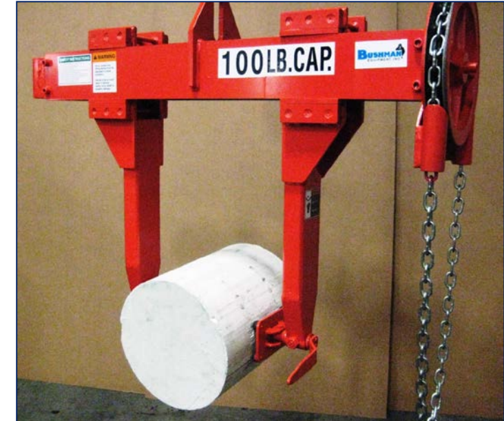
Lifter legs are operated with a hand chain wheel. Rotation is by a hand lever with locking detents.
