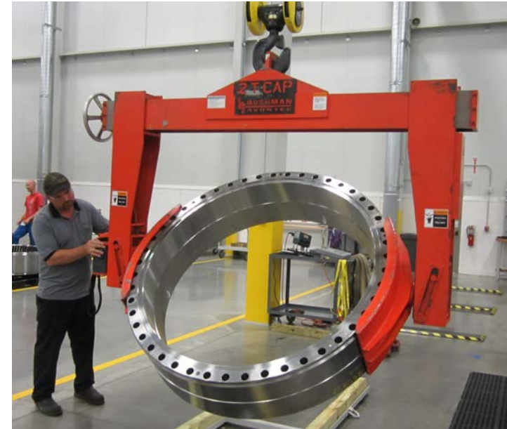
Grab uses end effectors with retaining lips for added security when lifting repetitive parts.
