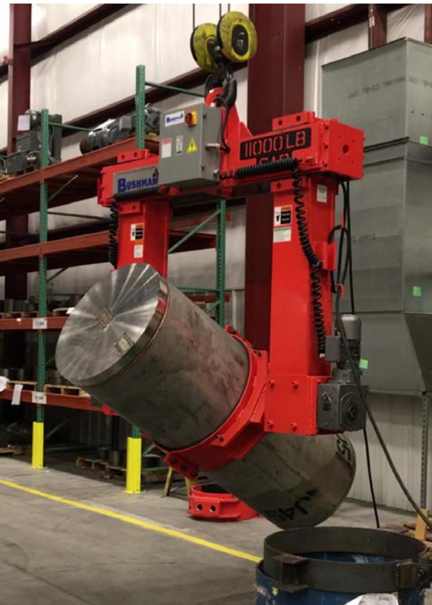
A clamp assembly attaches to a mixing cylinder. Each leg uses two pins to mate with the clamp assembly, allowing a safe lift and rotation.
