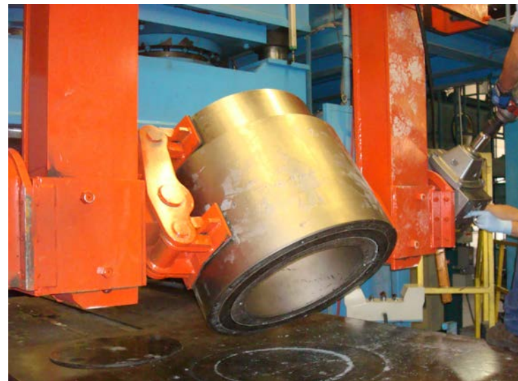
Inner and outer mold halves can be lifted and rotated during the molding process. Leg movement and rotation are by an air powered wrench.
