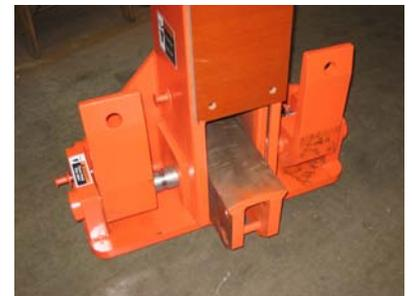
Coil lifter down, pallet forks up
