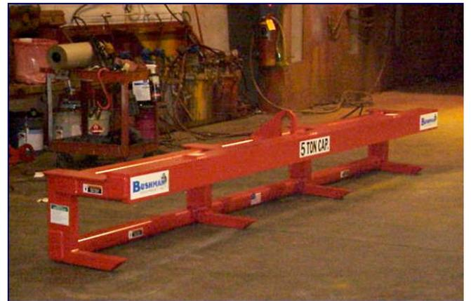
Pallet lifter modified to lift billets
