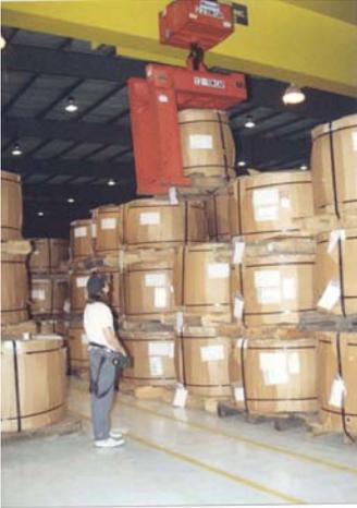
Bushman builds higher capacity pallet lifters with a double vertical member.
