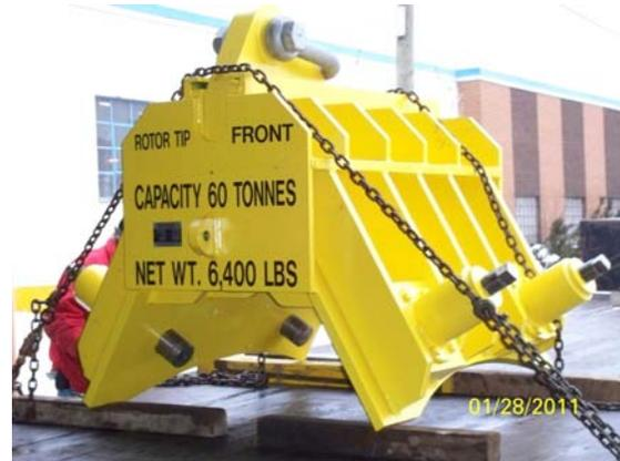
This is a special lifter for picking up nose cones with three blades during the installation of 2.5 MW wind turbines.
