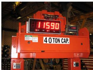
A major steel company is using coil grabs with built-in weigh systems to reduce product handling. They found these lifts save time and reduce product damage compared to their old procedure that used a floor scale for weighing.
