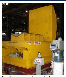
While moving through the process bay, coils are often placed on a floor scale and then on the upender. By including a load weighing system in your upender, you can upend and/or rotate coils and weigh them simultaneously. This reduces handling time and minimizes damage to the product. Using multiple load cells in the base of the upender, the signals are summed and a stabilized weight is displayed, unaffected by the motion of the upender.
