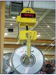
Bushman bottom blocks incorporate 360 degree, manual or powered rotating crane hooks that permit the crane operator to position heavy or awkward loads in less accessible work areas. Our unique design does not increase the overall height of the bottom block, an important feature for buildings with low headroom. The load weighing equipment is mounted directly on the bottom block to reduce EMI/RFI (electromagnetic or radio frequency interference).
