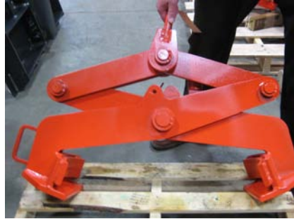
This supporting tong has a locking pin.
