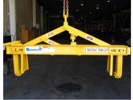
This three-ton supporting tong lifts rolls of steel belting.
