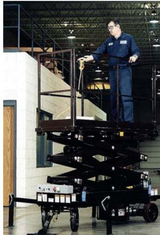
These 1,000 pound, hydraulically operated aerial maintenance lifts are dependable, affordable and generally maintenance free. They can pass through 36-inch doorways and fit into standard elevators for use in multi-story buildings. In spite of their high capacity, they are light weight and easy to transport between work sites.
