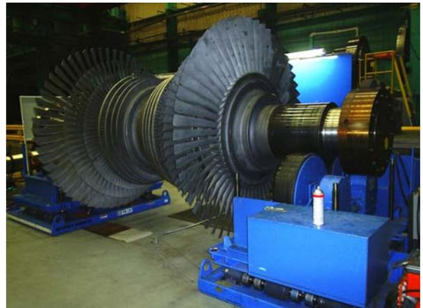
These twin arbor lifts can handle 60 ton turbine shaft assemblies. One lift is stationary while the other moves on air bearings to adjust to the shaft length. Both lifts rise to the desired work height on screw jacks.
