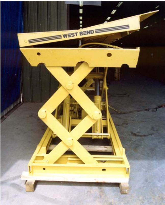
This coil discharge hydraulic lift table features a hydraulically operated top platform that lifts, lowers and discharges rolls to one side.
