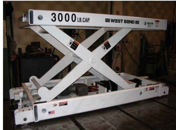
The STX-SCR scissor lift table uses a mechanical screw, driven by an electric gear motor, to raise and lower the platform. This table is designed for applications where hydraulics cannot be used or for extremely precise load positioning.
