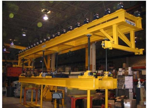
This 8,000 pound capacity lift has a platform that is 24 feet long and 54 inches wide. Its 68-inch vertical travel is made possible by six screw jacks that are all powered by a single 40 HP electric motor.
