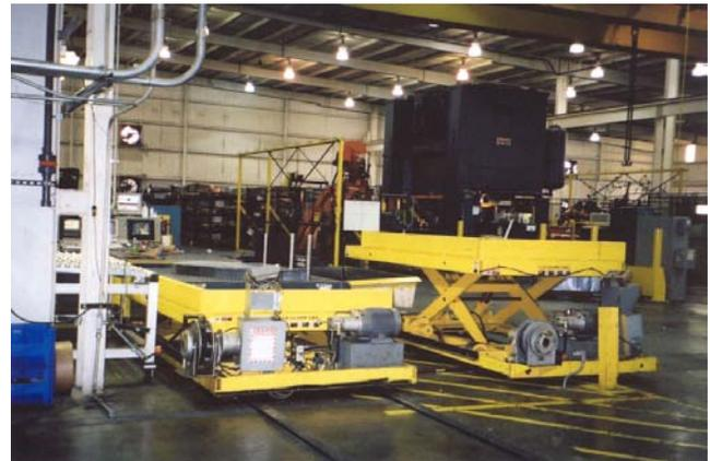
These 15,000-pound capacity traveling scissor lift tables are rail mounted. They provide an ergonomic solution for feeding material in a steel blanking facility. The scissors function permits the platform to index down as the stack height builds.
