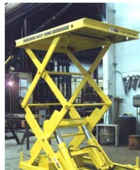
This double-high hydraulic scissor lift table allows extended vertical travel with a compact platform length. It is ideal for applications such as sheet-stacking and transferring materials between different levels in a building.
