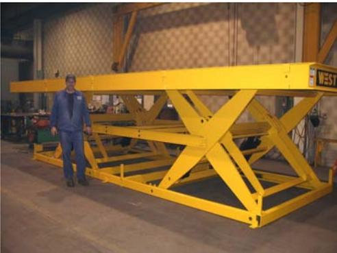
This custom double long scissor lift is used by a major flooring manufacturer to index sheets of linoleum flooring.
