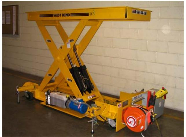
A nuclear facility project in Washington State recently ordered several highly engineered scissors lifts including a 9,000-pound capacity triple high lift cart and three 4,000-pound capacity high scissors lift extraction carts.
