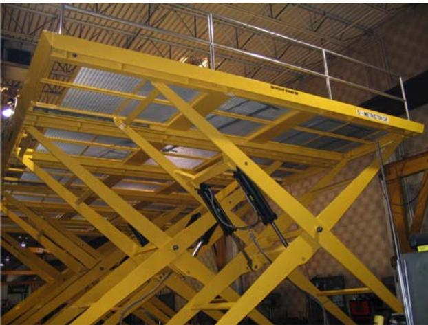
This 12,000-pound capacity scissor lift table platform is 23' x 44' and is used in a commercial jet engine test cell.
