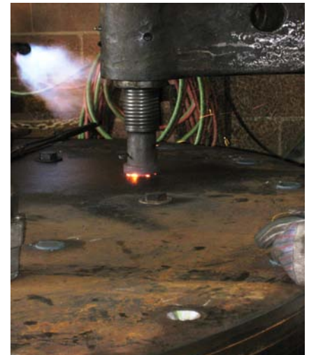
#6 Rivet is punched using the riveting machine.
