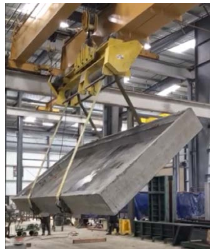
Flip-Rite® is used in many precast concrete plants.
