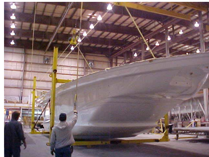
Using fixtures, irregularly shaped fiberglass boats can be safely flipped.
