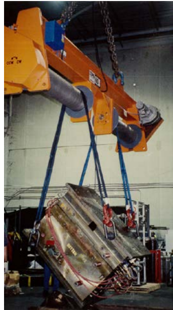
Using swivel hoist rings, a Flip-Rite® is used to tip from vertical to horizontal for mold maintenance.
