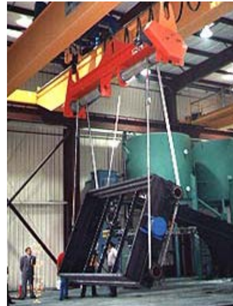
Flip-Rite® used to dump sand out of foundry mold boxes.
