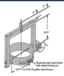
The Model 771 is a heavy duty drum tilter designed to manipulate drums in high production areas.
