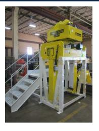
Because coil grabs are large and top-heavy, a properly designed storage stand is recommended. It can be designed for storage only or as a full maintenance platform and to aid in attaching the grab to the crane hook.
