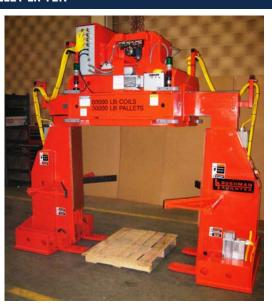
This combination coil-pallet lifter handles coils both eye-horizontal and eye-vertical on a pallet. In this application the lifter loads the coil eye-horizontal onto a coil tipper. While the coil is tipped onto a pallet, the grab "changes state" so it can pick up the palletized coil.
