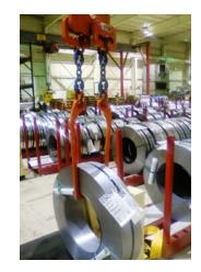
This lifter easily handles densely packed slit coils. It can deposit and remove slit steel coils (down to 1" wide) that are closely stacked in floor racks. The adjustable coil lifter has lifting legs that fit between the coils and rotate into the ID for a safe lift.
