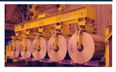
Above- Five (5) 20-ton coil grabs attached to a lifting beam to lift five coils simultaneously.
