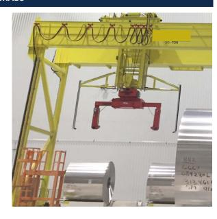
Bushman coil grabs are applied to fully automated overhead cranes used for coil movement & storage applications. Through collaboration with the crane OEM or system integrator, sensors are added to the grab to detect leg position, rotation position, presence of the coil or other obstructions. Signals are transmitted to the crane controller to either permit safe crane movement or prevent motion if an unsafe condition is detected.
