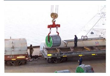
This 25-ton capacity adjustable coil lifter uses highstrength steel hooks to offload steel coils from a railroad car. Hook spacing is manually adjustable to match the coil width being lifted.
