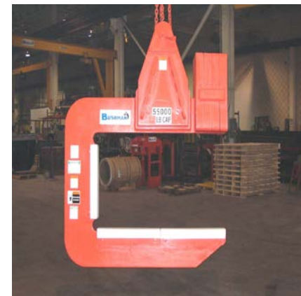
UHMW (Nylon) bolt-on pads
