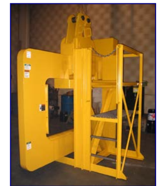
Platform helps with attachment to crane hook
