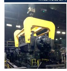
Mill roll lifters are offered in various configurations for lifting one roll or a two-roll set. Capacities up to 100 tons. Manual lifters include flip-down lifting pins (shown at left) or a tong-style lifter (above). Motorized designs are also available
