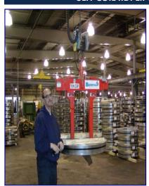
I.D. coil lifters are used to handle slit, banded coils from a packaging line and load onto pallets. Lifting pads are lowered through the I.D. and then opened to lift from under the coil. These lifters are operated by either a hand wheel or through an electric motor.
