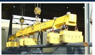
Magnet beams feature twin bail lift-up, fixed length or our motorized telescopic Tri-Beam™, and hardened steel bushings at magnet attachment points. Beams are available with built-in storage stands.
