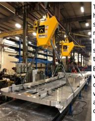
The FLIP-RITE® material handling system allows safe raising, lowering, rotating and leveling of large, bulky or oddly shaped objects up to 100 tons. The FLIP-RITE® gently rotates heavy loads within the envelope of conventional lifting straps without the shock loading and wear & tear to your crane.
