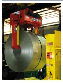
Motorized coil grabs are a fast, efficient way to handle coils. They are custom-designed to handle your heaviest coils and their full range of widths and diameters. Options include coil protection features, motorized rotation, weighing systems, automation, controls for AC or DC motors.
