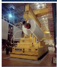
Manual or motorized rotating spreader beams allow the load to be rotated 90° or more from its pick-up position. Available options include position sensing, limit stops, weigh systems and motor controls.
