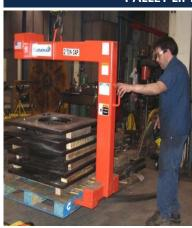
Bushman pallet lifters are available in capacities from 500 pounds to 20 tons. Pallet lifter features include:
