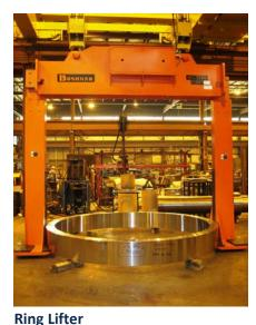
This unique lifter loads forged rings into and out of vertical turret lathes. It can lift rings from the OD or the ID.
