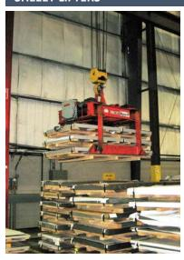
Sheet lifters handle single or multiple bundles of metal sheets or plates. They are operated by a hand wheel, chain wheel, electric motor or hydraulic cylinders. Options include extendable carrying arms, adjustable load forks, self-contained battery power systems, motor controls and much more.
