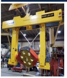
Rotating horizontal axis grabs grip the outside of a load and rotate it up to 360° to the proper position. They can be operated manually or powered by an electric or air motor.
