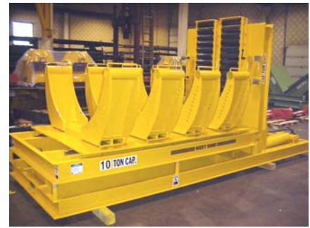
This hydraulic upender was designed for handling transformers.
