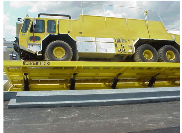
This hydraulic upender is a tilt-test table. E-One, a manufacturer of crash and rescue vehicles, needed to test their vehicles for stability when operating in rough terrain. Maximum lifting capacity of the table is 150,000 pounds and the maximum tilt angle is 40 degrees.
