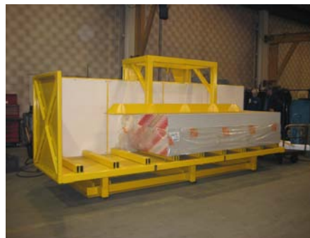
This hydraulic upender was designed to upend loads of drywall. The wall is incorporated into the left hand end of the upender to assist the forklift operator in squaring up the load. The loading deck of the load platform has removable fork guides. An electric powered clamping arm secures the stack while tilting.
