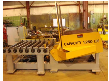
This is a custom upender designed to take coils of steel rod from the customer's forklift and lay them down onto a wire mesh pad for transport through the customer's annealing furnace. The unit has two "wings" that are actuated simultaneously to center the coil of steel rod onto the mesh pad on the conveyor section.
