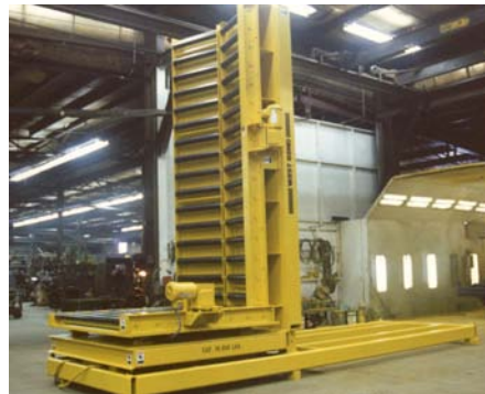
This Bushman hydraulic paper roll upender is designed to palletize loads of laminated paper or other materials.
