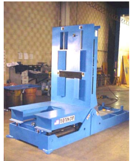
This upender has a powered V-saddle and a clearance slot for the C-hook used to place steel coils onto the V-saddle.
