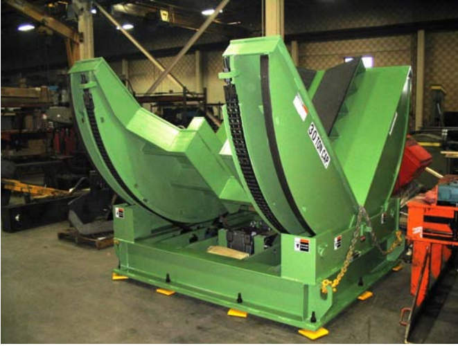
This 30-ton mechanical upender was designed for a steel mill.
