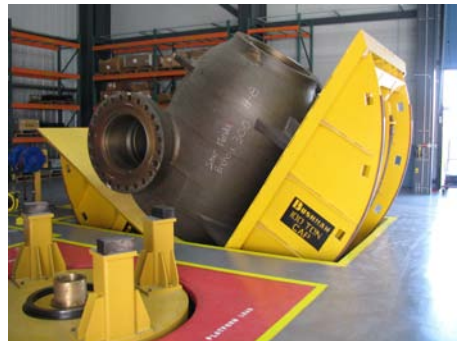
200,000 pound capacity mechanical upender mounted in a pit so that platforms will be level with the floor. Upending time is approximately 45 seconds.
