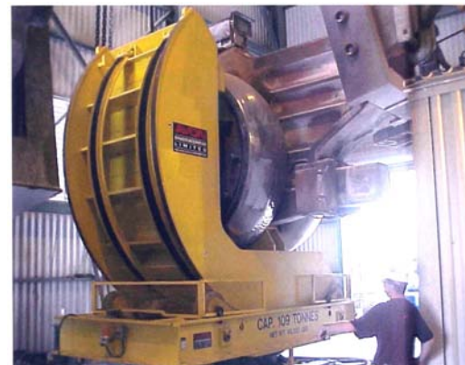
109-metric ton mechanical upender has a motorized rotating base.
