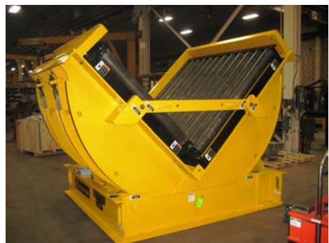
This 60,000-pound mechanical upender has gravity roller conveyors on both platforms plus a diagonal locking bar to secure the mold while it is on the conveyor.
