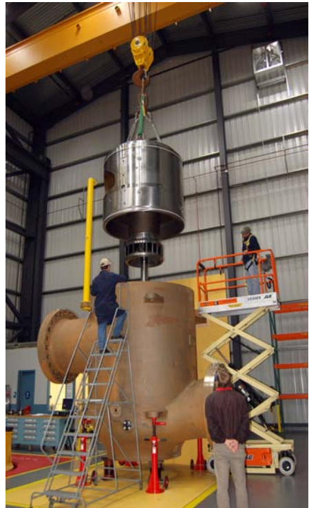
This 100-ton capacity mechanical upender is used to assemble a gas compressor.
