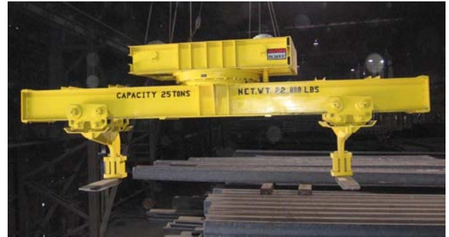
25-ton capacity spreader beam with powered rotation and lifting forks with adjustable spacing for handling hot beam blooms.
