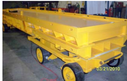
60,000 pound capacity towable tube bundle cart. This cart has a hydraulic braking system.
