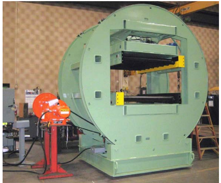
Hydraulic barrel inverters, named for their circular shape, are suited to high capacity or high volume operations.
