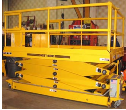
7,000 pound capacity triple high scissors lift platform.
