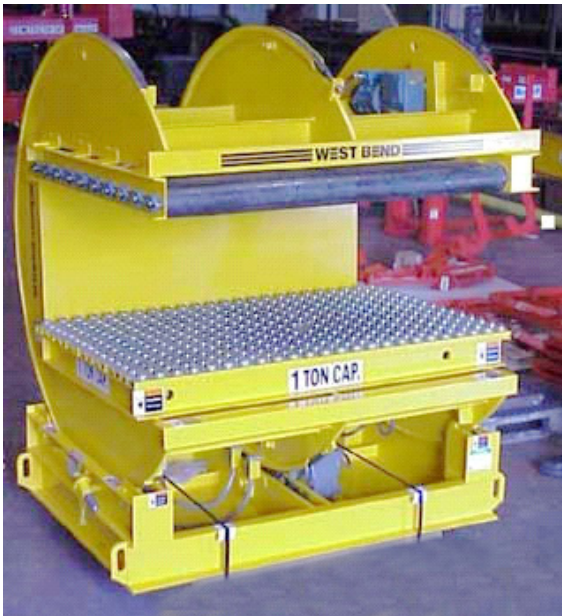
C-frame inverters have a C-shaped cradle that can handle long loads that may extend beyond the end of the frame.
