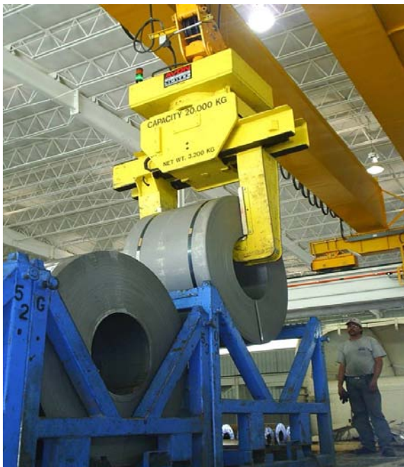
This motorized rotating coil grab was designed for low headroom areas.
