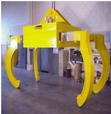
**Custom 70,000 lb capacity grab has four legs that open and close on a circular-plate electrode simultaneously, ensuring that equal pressure is applied to the entire outside diameter.**
