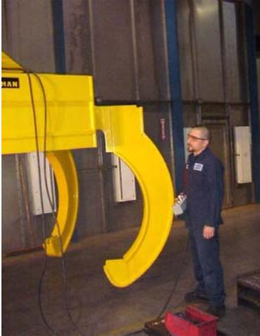
**Lifting grab is designed to withstand high temperatures inside electric steel furnace. Its legs are operated remotely as the grab secures and lifts bottom electrode in furnace without human intervention.**
