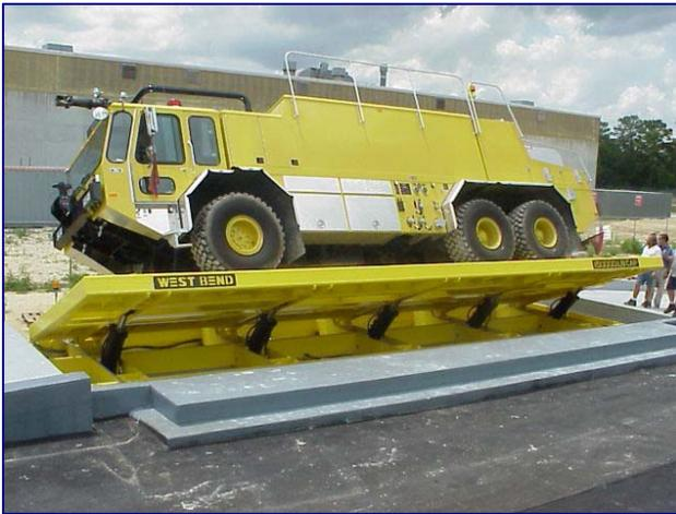
During a test, the truck is driven onto the table, and its axles are secured with chains. The truck is then tilted to the point when the tires begin to lift off the table. This position determines the rollover threshold that is recorded.
