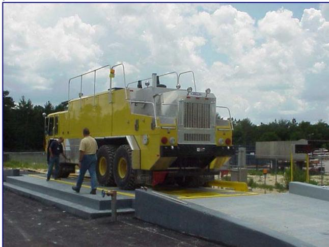
The base is a two piece weldment, and the tilt top that the truck drives onto is a separate piece. These two pieces were hinged together on the 40 foot side. Tilting is accomplished by five, 7 inch diameter dual acting hydraulic cylinders,
