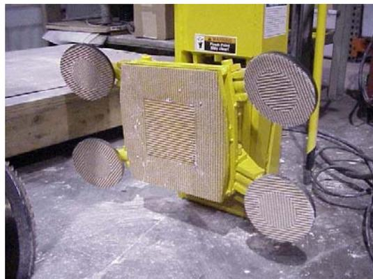
**This Model M2038 motorized rotating axis grab has a capacity of 3,000 pounds. It was designed to lift and rotate graphite blocks from six to 20 inches wide. The blocks are 42 to 70 inches long.**
