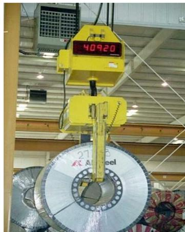
***Bushman AvonTec Coil Lifter Equipped with a***
