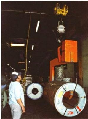
***Typical Below-the-hook Lifting Equipment***
