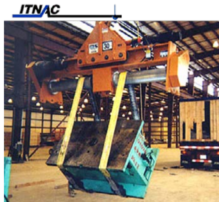
ITNAC Flip-Rite™ used to rotate a stamping die. This unit also has the Level-Rite™ lifting bail to ensure a level-lift of an unbalanced load.
