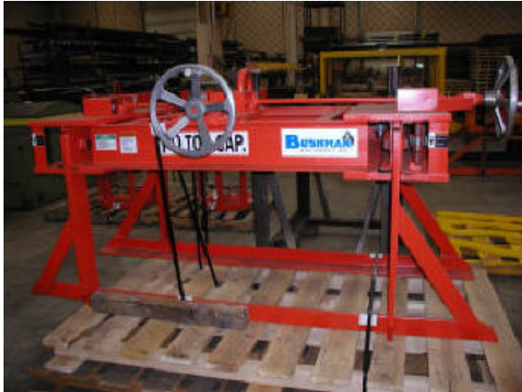
Manual sheet lifter with dual operation hand wheels
