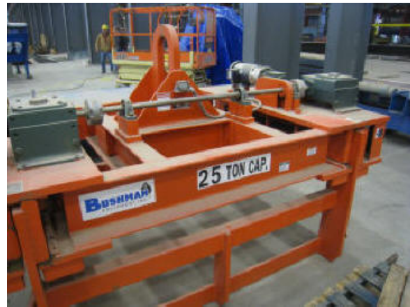
25-ton motorized sheet lifter ready for service
