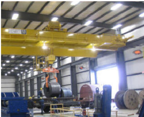
55-ton, Model 427, Adjustable Coil Lifter
